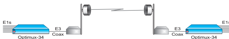
E1 fan-out over radio links
