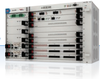
Gmux-2000, modules view
