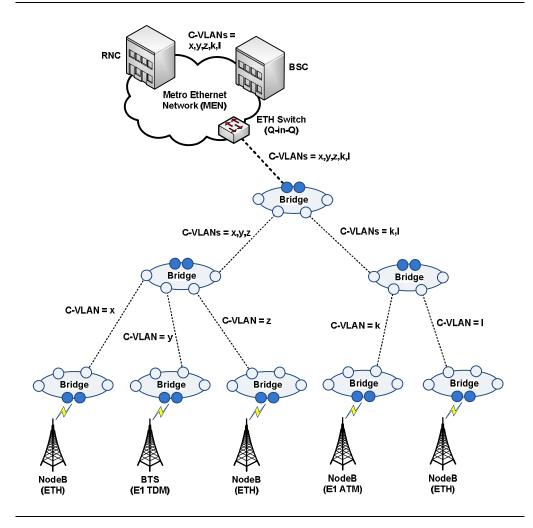
**Description** Ethernet frames from all the BSs are forwarded to an Ethernet Switch, which adds/ strips an S-tag for each individual C-VLAN.
