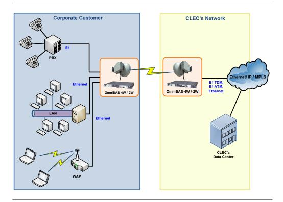
**Description** OmniBAS incorporating efficient bandwidth handling mechanisms allows excessive bandwidth to be leased to corporate customers needing economical high-capacity permanent connections.
