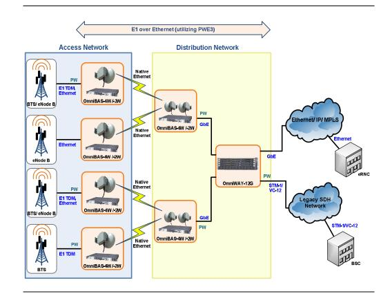
**Description** OmniWAY aggregation platform fully complements OmniBAS PtP product family. Mobile operators can implement nodal configurations for aggregating packet-based traffic from multiple OmniBAS systems and provides connectivity toward the Ethernet network (Ethernet/ IP/ MPLS), through GbE interfaces, or toward the legacy SDH network, through STM-1 (VC-4 and VC-12) interfaces
