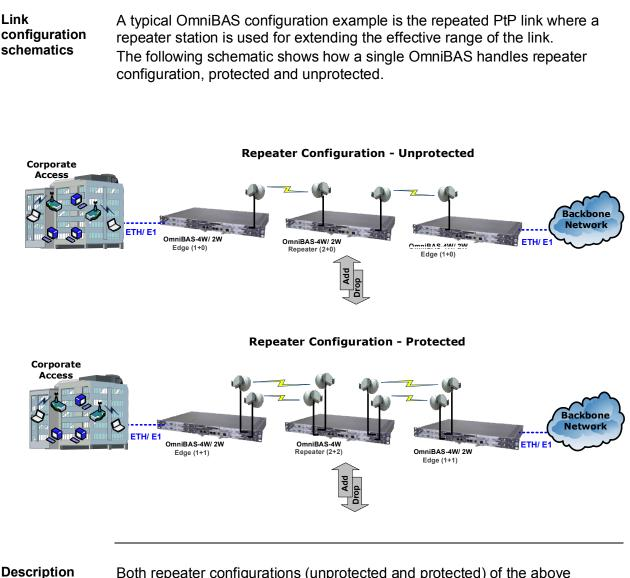
**Description** Both repeater configurations (unprotected and protected) of the above examples, depicts three OmniBAS systems that are used to transport legacy E1 and Ethernet traffic from a corporation toward the backbone network. In the *unprotected repeated configuration*, the two OmniBAS-4W/ 2W systems at the edges of the link are configured for 1+0 operation, while the third OmniBAS-4W/ 2W system at the repeater station is configured for 2+0 operation.
