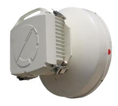
About ODU-CF OmniBAS system provides a complete family of ODU-CF units covering a wide range of operating frequencies: 6 / 7 / 8 / 11 / 13 / 15 / 18 / 23 / 38 GHz. The ODU-CF incorporates the radio transceivers featuring capacity up to 400 Mbps. It supports adaptive modulation schemes from QPSK to 256 QAM and channel bandwidths from 7 MHz to 56 MHz. The capacity and modulation agility is achieved without the need of hardware change.
