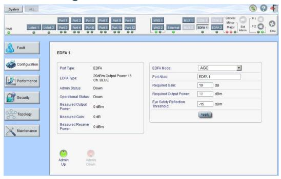
Figure 99: EDFA Configuration Window
