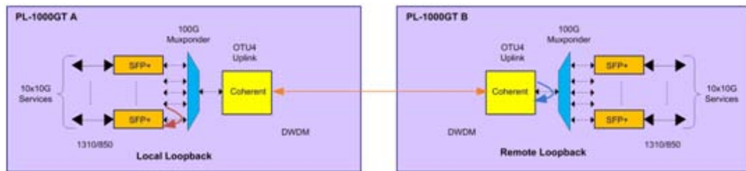
Figure 136: Facility Loopback Test
