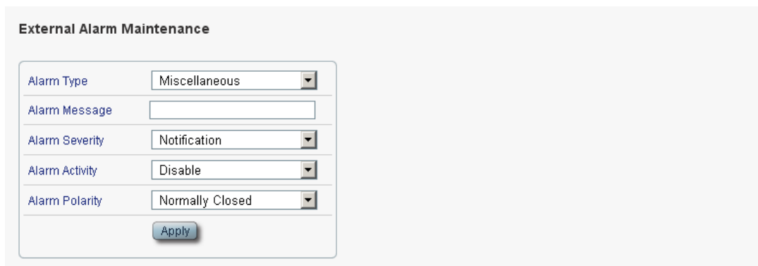
Figure 146: External Alarm Tab
