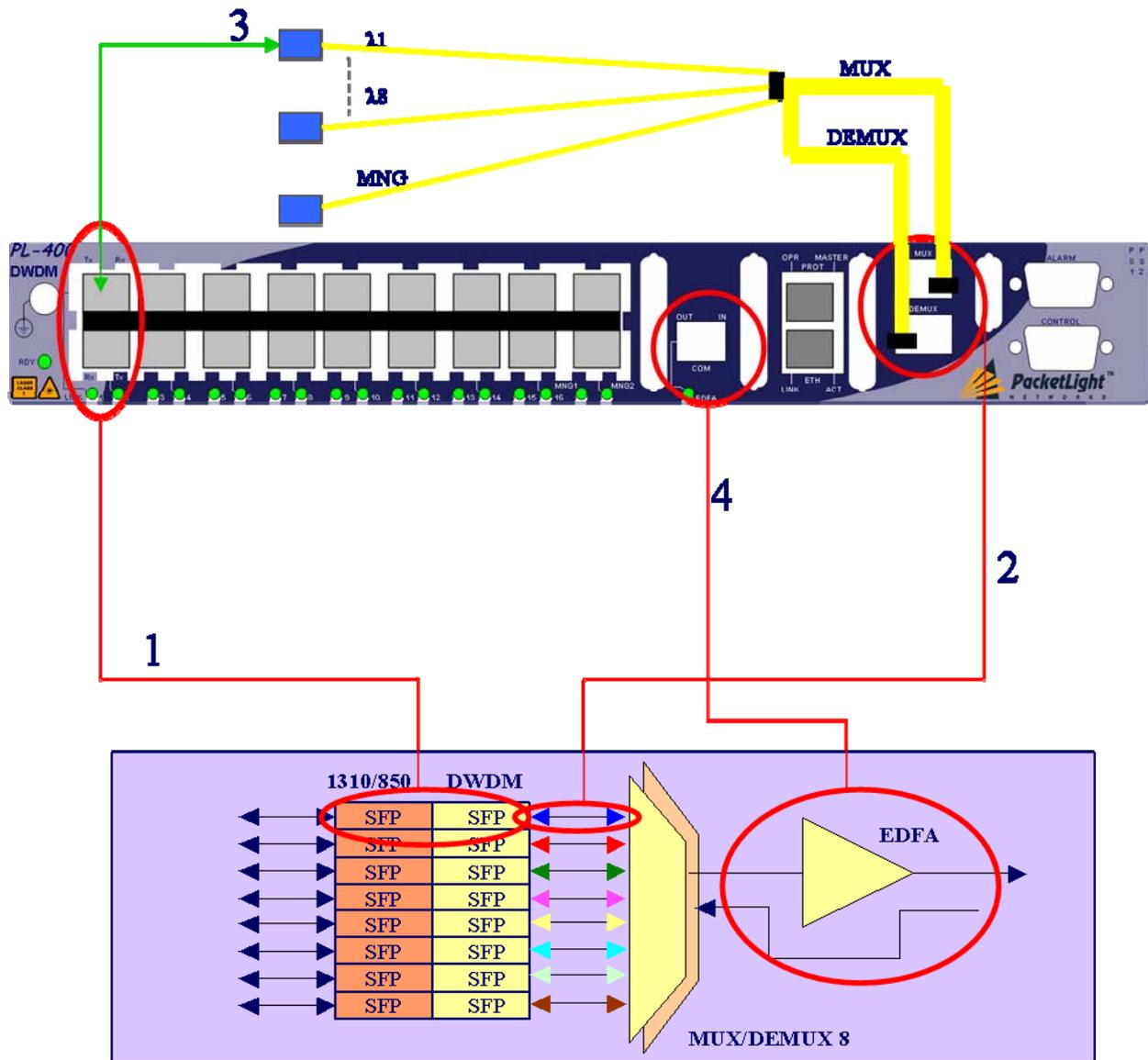
Figure 2-3. Connections between Optical Interfaces
