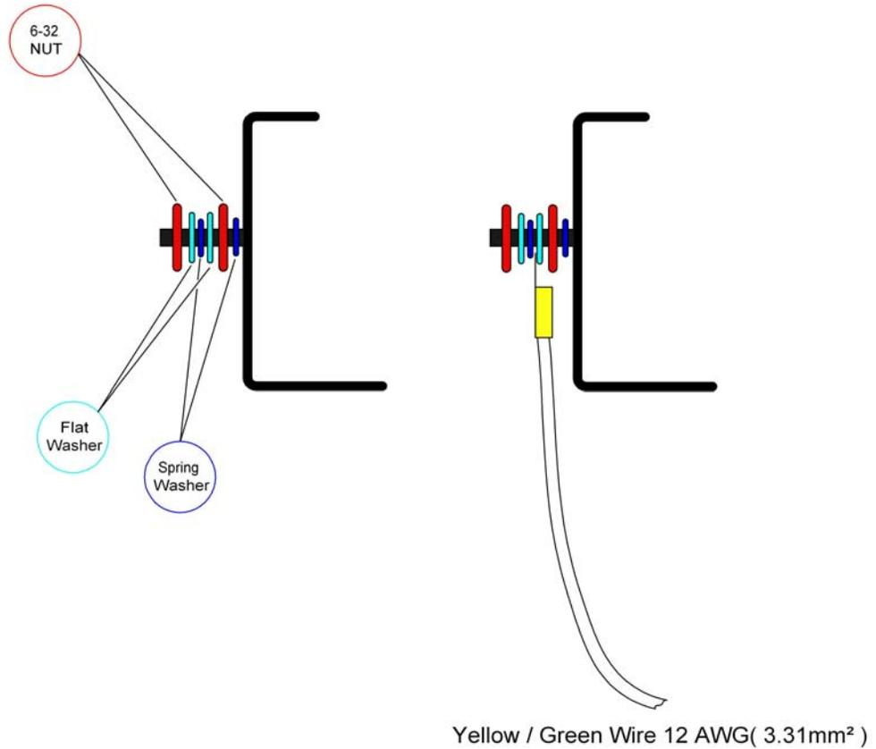
*Figure A-3. Protective Ground Terminal Wiring Diagram*
