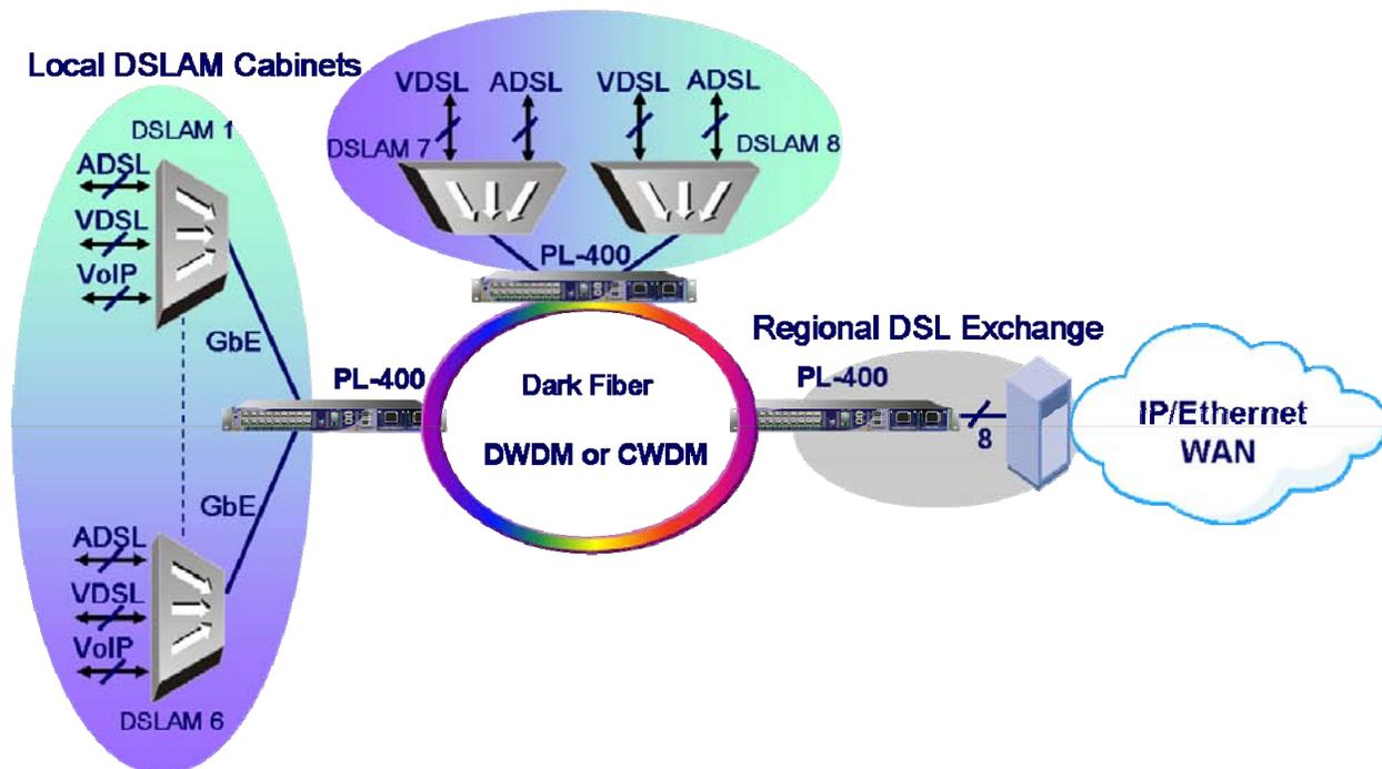
Figure 1-13. DSLAM Ring Application for PL-400 Devices
