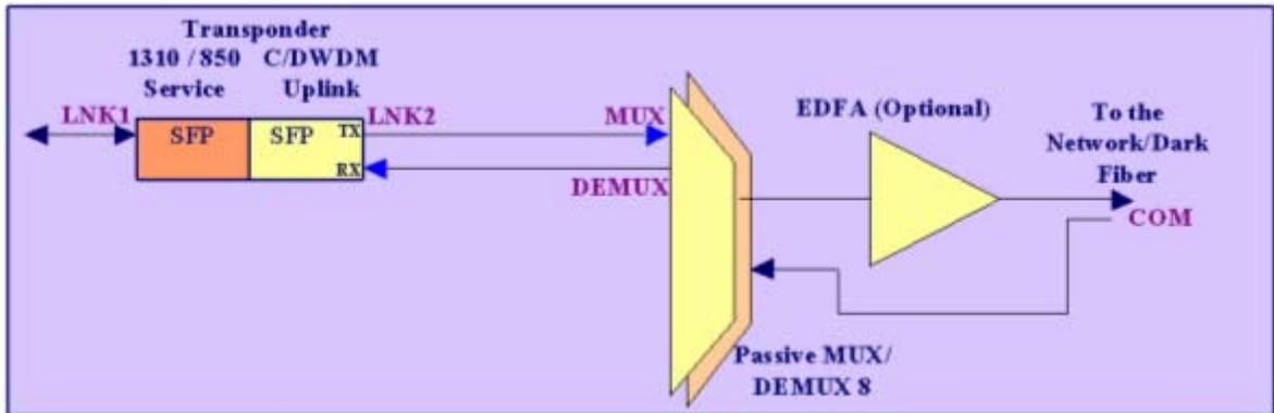
Figure 2-4. Connections and Naming of Optical Interfaces
