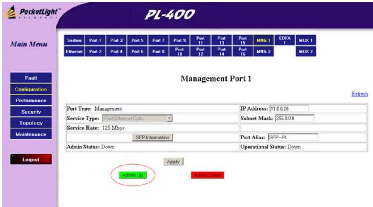
Figure 4-11. Configuration: Enable a Selected Port
