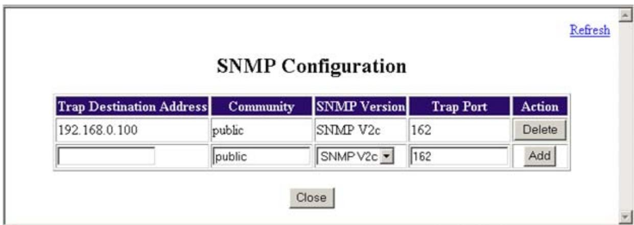
Figure 4-2. Configuration: SNMP Configuration Window
