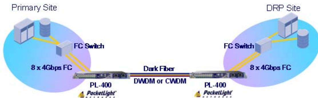
*Figure 1-12. Typical Storage Application for PL-400 Devices*
