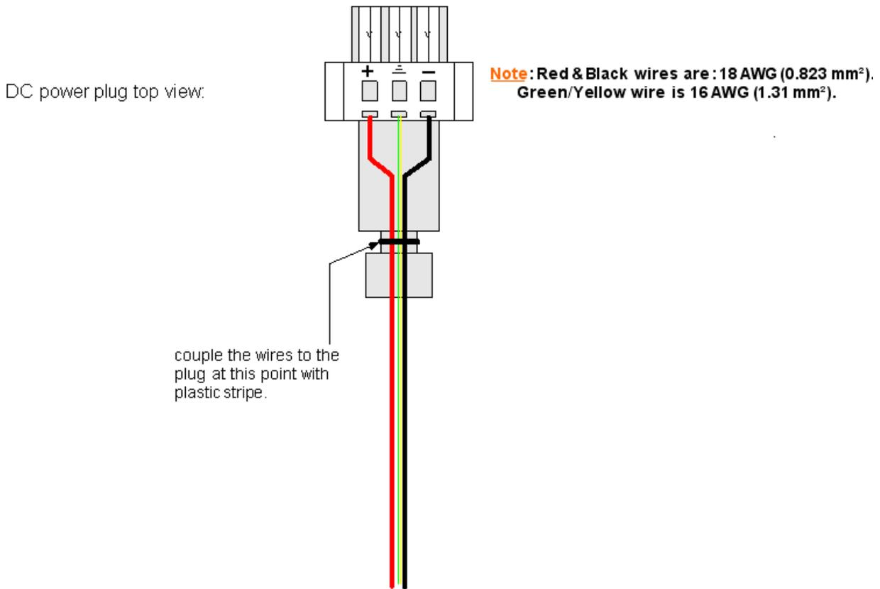
Figure A-2. DC Connector Wiring Diagram
