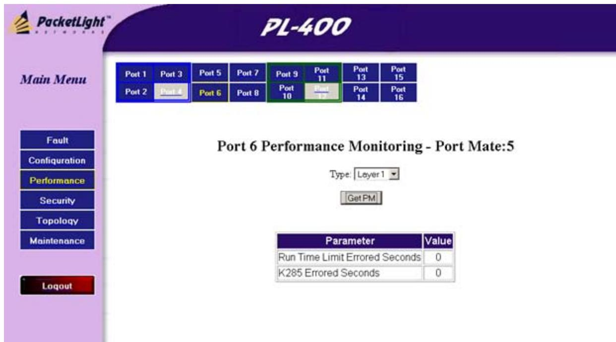
Figure 6-4. Performance Monitoring: Layer 1 Errors
