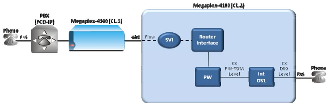
In order to transfer voice traffic through a Packet Switching Network, MP-4100 should first convert PCM voice signal to ETH flow.
