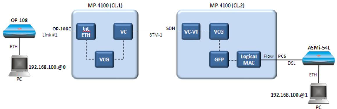
The Packet (Ethernet) Engine of MP-4100 is a state-of-the-art, multi-port GbE switching and aggregating block, which enables hardware-based Ethernet capabilities, such as traffic management, performance monitoring and OAM, between any of the Ethernet entities.
