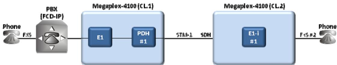
In order to transfer voice traffic through an SDH Transport Network, analog or digital voice channels should be assigned to the corresponding E1 channels and then mapped to STM-1 frame.
