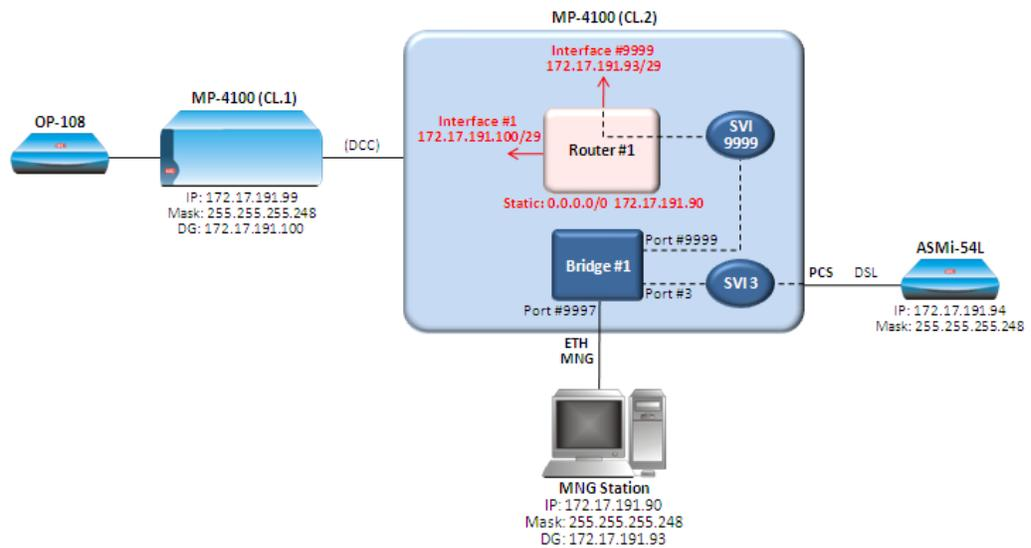
Management station is connected to MP-4100 CL.2 via ETH-MNG port of CL-A.
