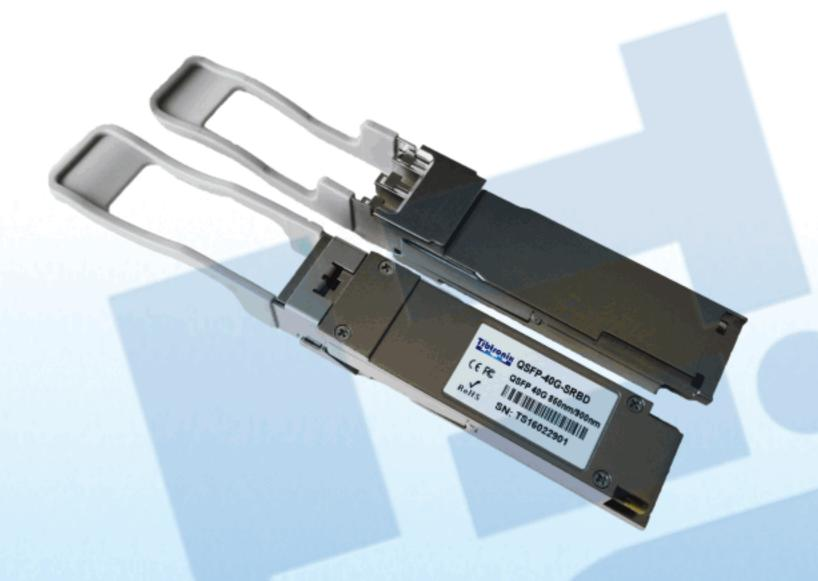
40Gb/s QSFP+ SR BiDi, Duplex, LC Connector, Hot Pluggable, 850/900nm, 100m on OM3 fiber, or 150m on OM4 fiber, VCSEL, Multimode
