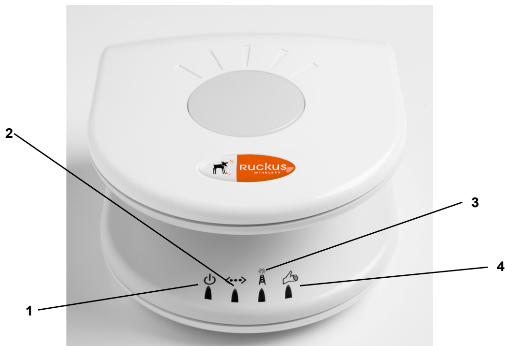
Figure 7—Front view of the Metro Broadband Gateway
