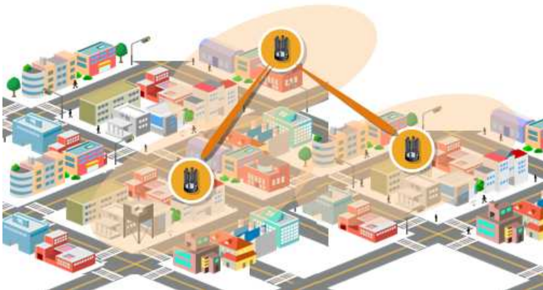
Figure 3.11 Self Backhaul Configuration
